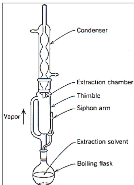
**Figure 2.3:** Soxhlet extractor diagram
