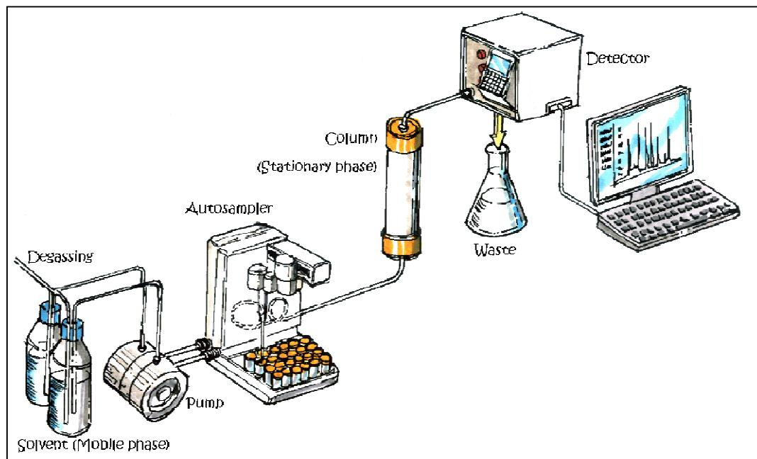
**Figure 2.5:** High Performance Liquid Chromatography
