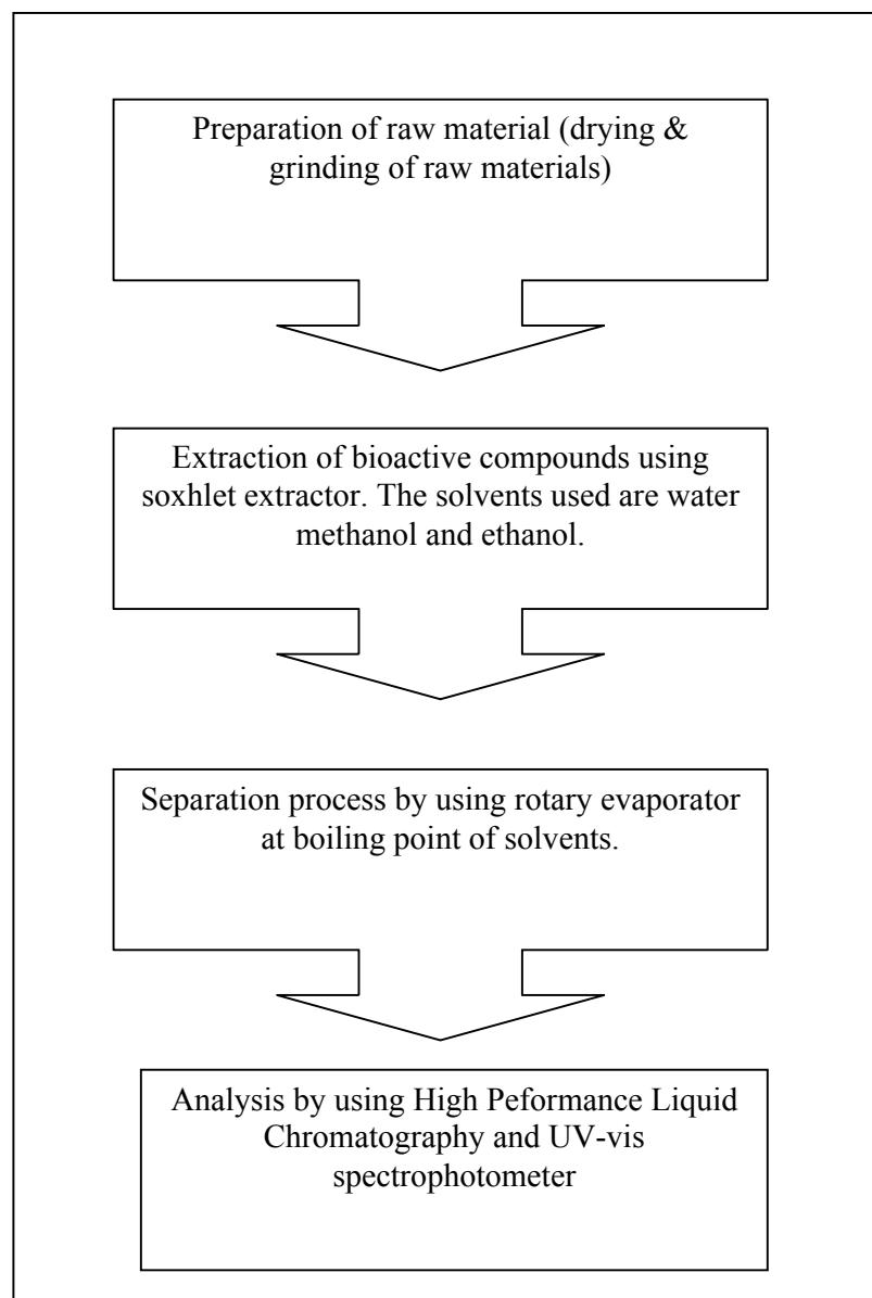
**Figure 3.1:** Process flow diagram
