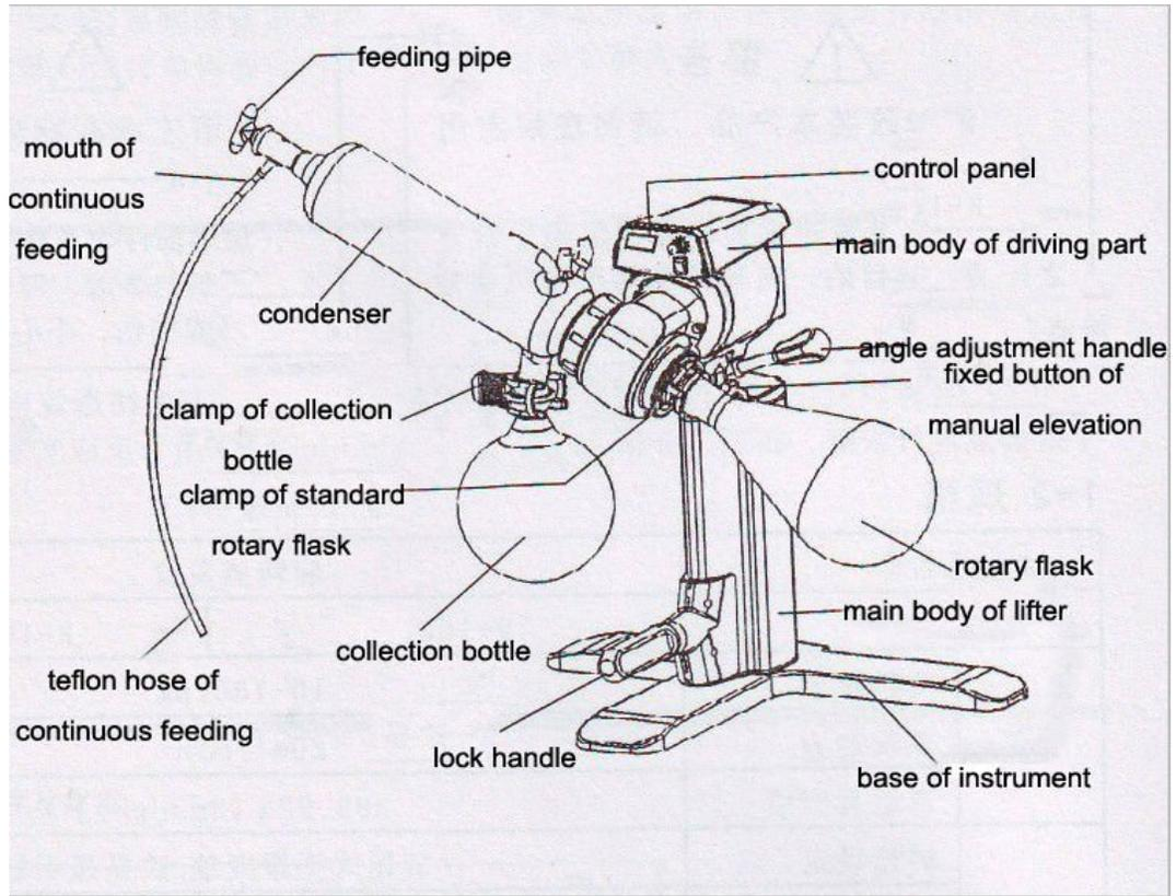
**Figure 2.4:** Rotary evaporator.
