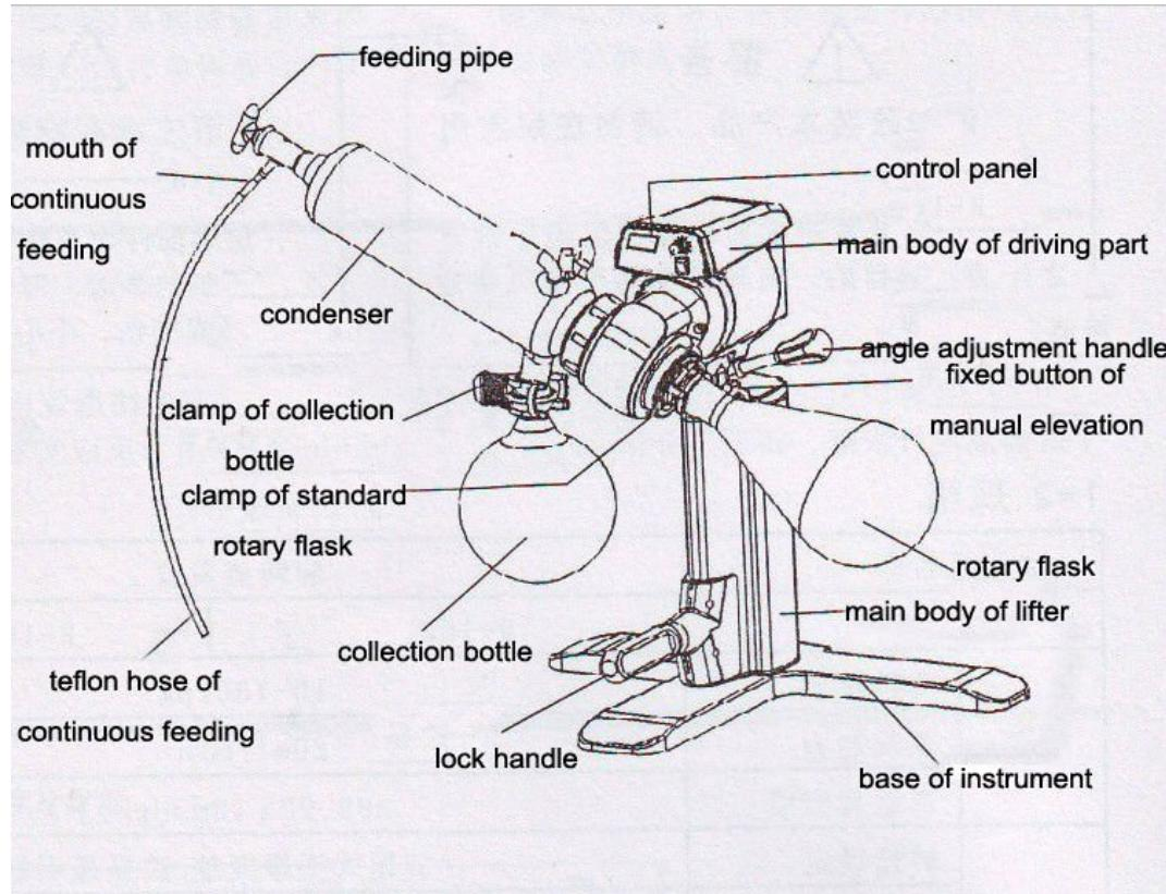
**Figure 2.4:** Rotary evaporator.
