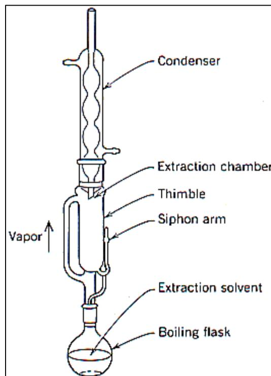
**Figure 2.3:** Soxhlet extractor diagram
