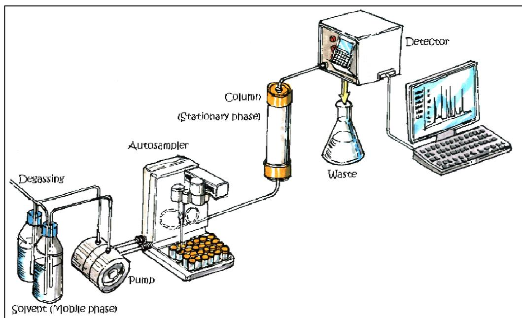
**Figure 2.5:** High Performance Liquid Chromatography
